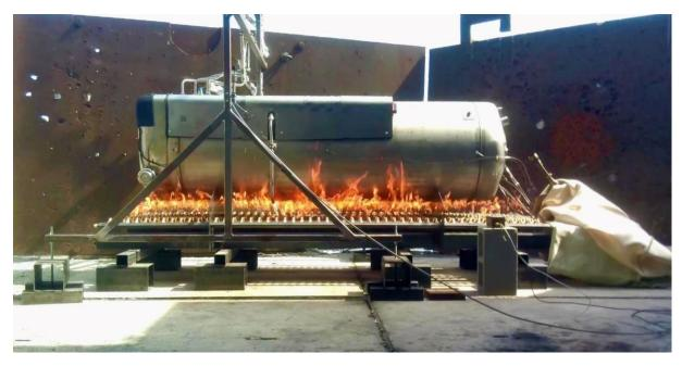
The liquid hydrogen tank system for trucks developed by SAG Group (www.sag.at) has reached a last milestone on the way to approval for road traffic
