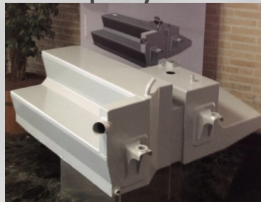
Low-entry bus diesel tank (mounted partly under entry)
